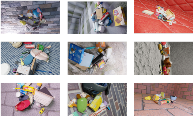
Figure 9. Example images from the synthetic dataset generated with a physically based renderer (PBR).
